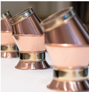
A binnacle – a housing for a compass that is installed on a ship's bridge
